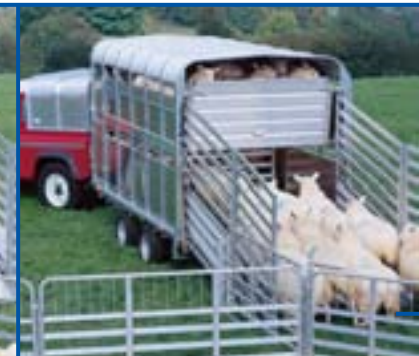
EasyLoad™ has been lowered and the lower deck is being loaded.
