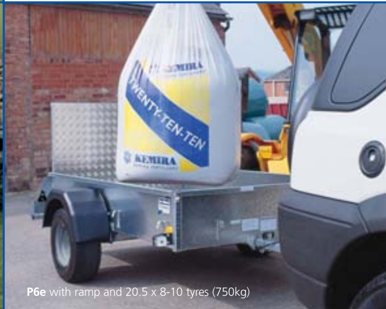
P6e with optional stock ramp door, weldmesh panelled sides and 20.5 x 8-10 tyres (750kg)
