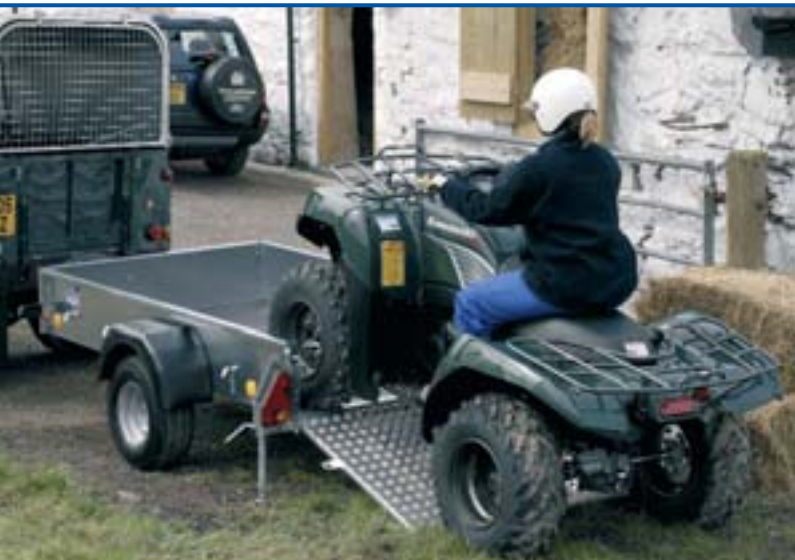
P7e with ramp, optional rear prop stands and 20.5 x 8-10 tyres (750kg)
