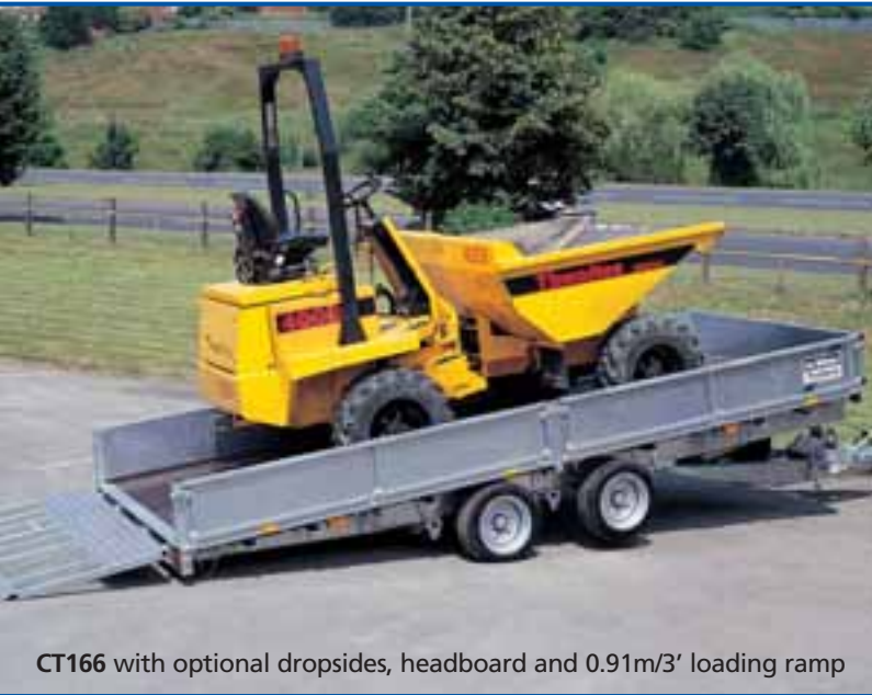
CT166 with optional headboard and 0.91m/3' loading ramp
